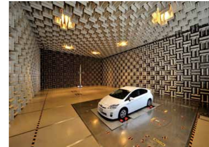
Electromagnetic Anechoic Chamber
